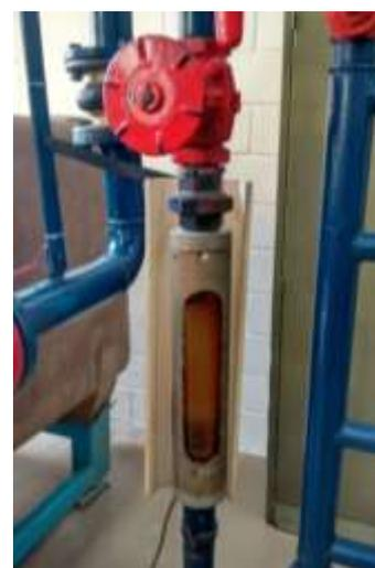
**Figure 5.** Rotameter coupled to the circuit.
