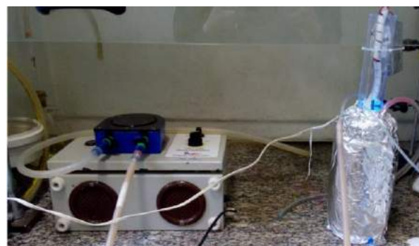
Figure 1. Photo of the vertical reactor used in the experiments: a) peristaltic pump and b) vertical reactor containing the UVC lamp (schematic).
