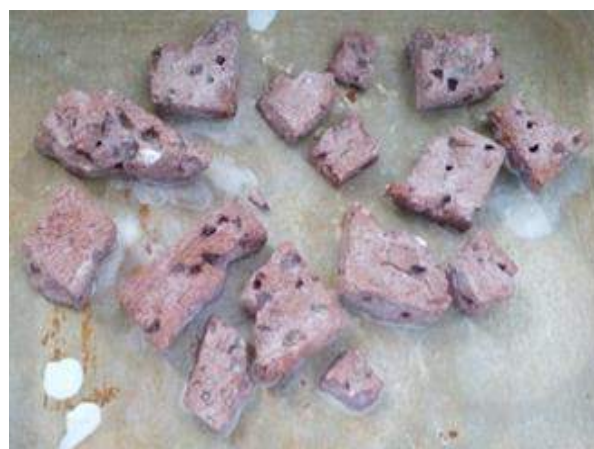
Figure 2. Ceramic samples impregnated with TiO 2 .
