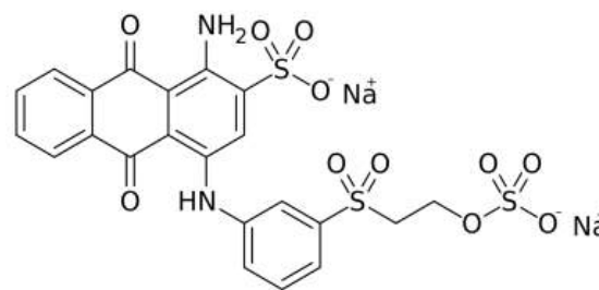
Figure 1. Chemical structure of Remazol Brilliant Blue R dye 16 .
