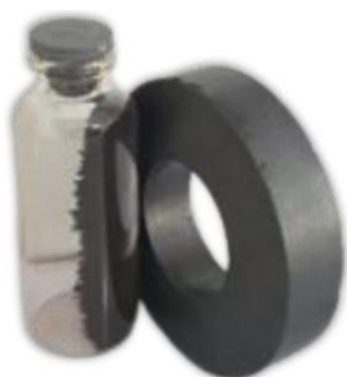
Figure 1. The application of Fe 3 O 4 /SiO 2 /C nanomagnetite by an external magnet.
