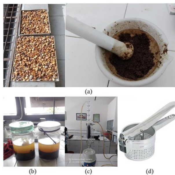
Figure 4. Students use the extraction method. (a) sample preparation (b) alcohol maceration; (c) soxhletization of n-hexane; (d) mechanical press.
