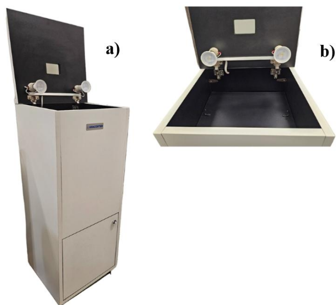
Figure 1. Imaging system (a) and the chamber where the sample is placed for taking the pictures (b). Note that the rectangular hole in the cover is where the smartphone is positioned after the cover is lowered.
